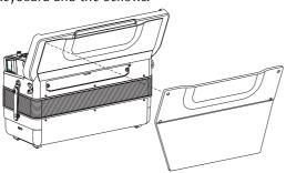
(4) Use the coin to loosen the two screws of the compartment cover.
